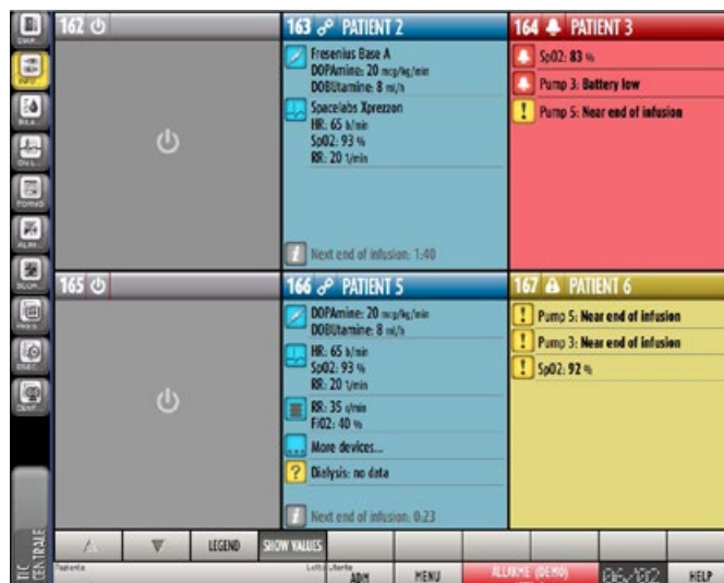
A sample screenshot of Digistat® Smart Central, showing 6 beds with patient vital signs from monitor, ventilator and infusion pumps including some alarms and warnings.
