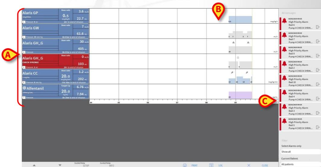
On the left, each box represents a pump. These boxes are named “Pump buttons”. The pump button displays the drug name when the pump provides this kind of information. When it doesn’t, the pump name is displayed.
