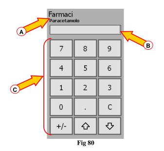
The name of the selected item is displayed above the keyboard (Fig 80 A). The example shown in the figure displays "Farmaci (Paracetamolo)". It is the same item selected on the "Fluid Balance items" table (Fig 82). When another item on the table is selected the name displayed in Fig 80 A changes accordingly.
