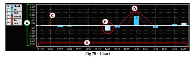
The variations in the fluid balance are represented by the blue vertical bars (Fig 70 **D** - the color is red when referred to blood changes, see Fig 73). The white line in the middle of the chart is the zero level (Fig 70 **C**). The bars above the white line represent fluid INs, the bars below the white line represent fluid OUTs.
