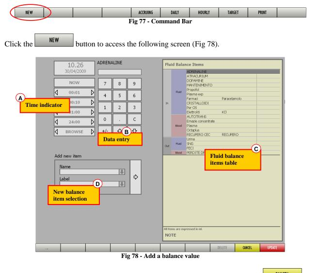
The screen is in "edit" mode, i.e. it is possible to edit the data displayed; the CANCEL and UPDATE buttons on the command bar are active.
