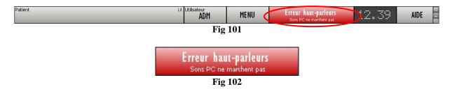
The notification remains while working with "Smart Central". It disappears when another "Sound Check" procedure is performed and a "YES" answer is provided in the end.
