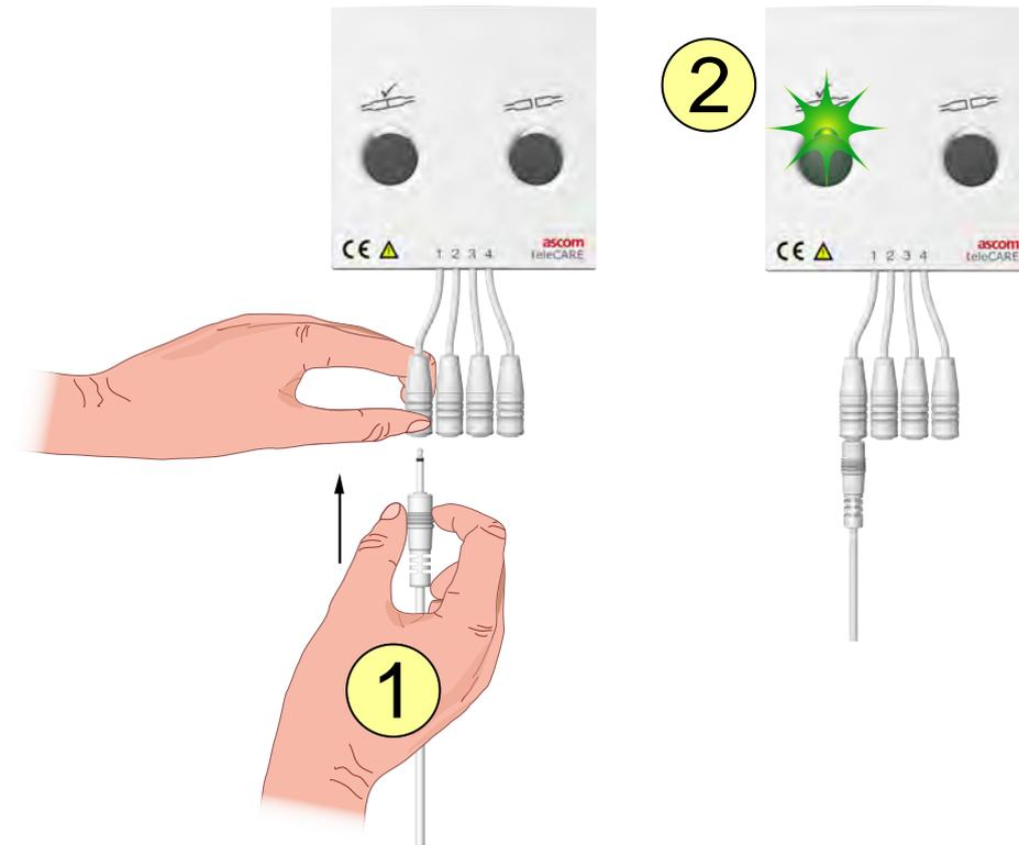
1. Reconnect the multi medical alarm cable to the required input.
