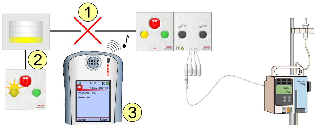
1. The multi medical alarm module fails to operate (broken, disconnected)
