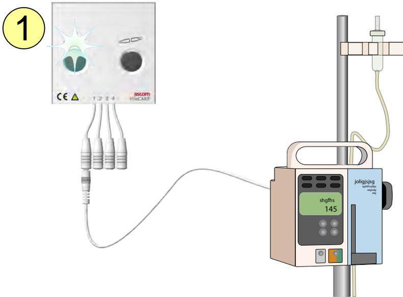
1. The multi-color LED above the test button will flash white if the system configuration for the multi medical alarm module is wrong, not existing or during a start up of the system.
