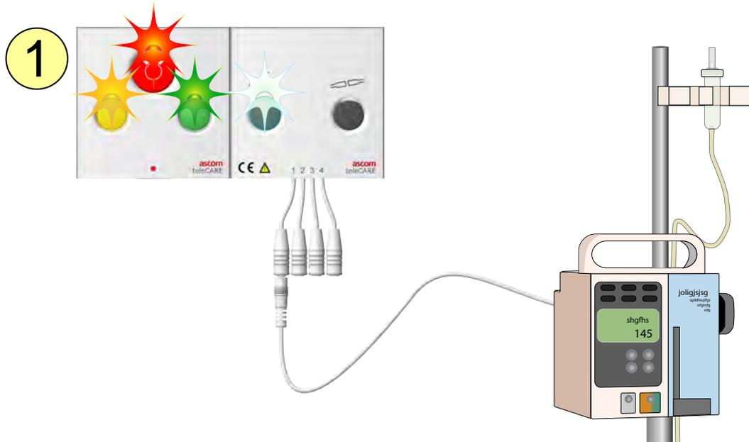
1. When the power returns, the multi color LED above the left button of the multi medical alarm module and all the LEDs on the bedside module will start flashing to indicate that the startup procedure is in progress.
