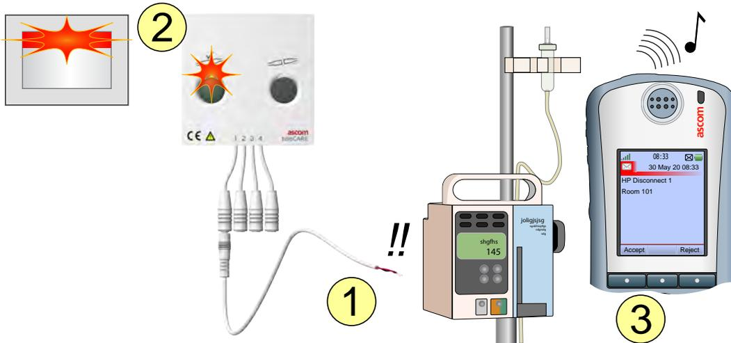
1. The multi medical alarm cable gets disconnected from the primary medical device by a loose contact or a cable break.
