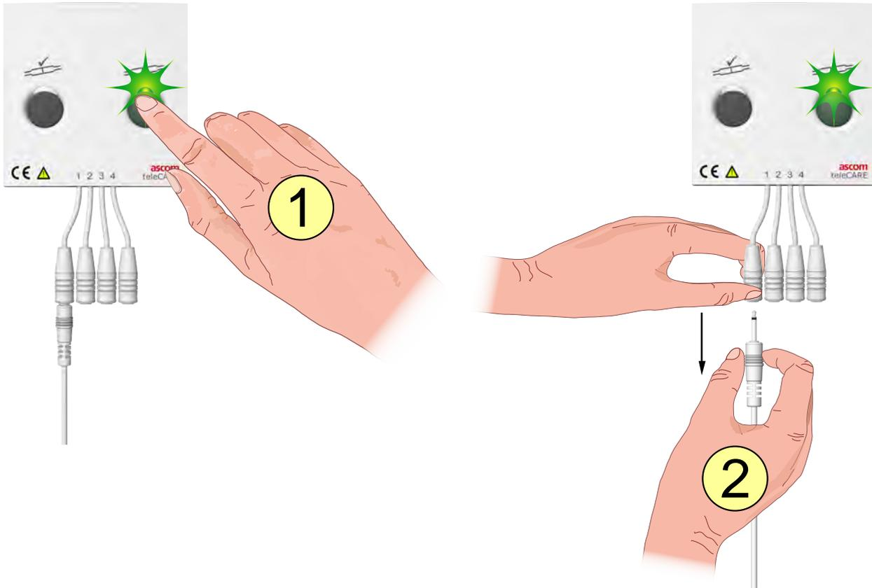
1. Press the “Disconnect” button on the right (green LED on).
