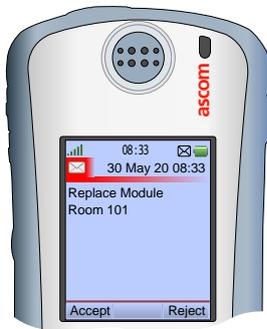
The input will still function normally but a proper connection to the primary medical device cannot be guaranteed. When continuing to use the worn input, the assigned technical personnel will receive a “Replace module” message for every 20 connections that are made to the worn input.
