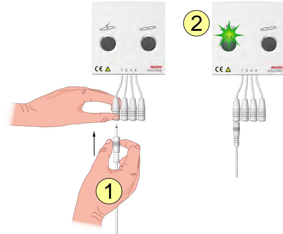
1. Insert the multi medical alarm cable into one of the four inputs depending on the messaging priority.
