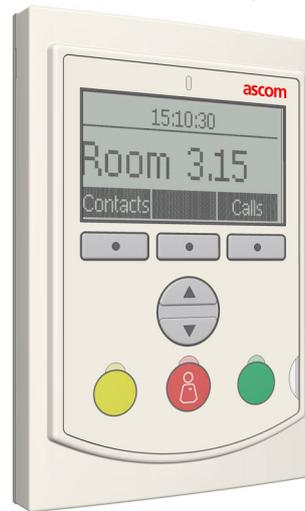
The Room Display module is similar to a bedside module; however, it has no sockets for beds and other equipment. The display is equipped with buttons and a loudspeaker for generating tones and buzzes. One room display can annunciate calls for a single duty area or an area equal to a staff console coverage area.
